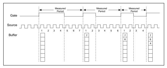
Figure 2-25. Buffered Period Measurement
